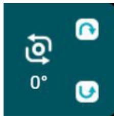
Use the **Rotate** control to rotate the camera display clockwise and counterclockwise in increments of 90°. rotates the camera display clockwise and rotates counterclockwise.
