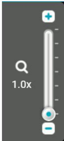
Use the **Zoom** control to adjust the level of zoom. Press the and icons to adjust the level of zoom in increments of .1x, between 1x and 6x. Zoom can also be adjusted using the slider by left-clicking on and dragging the mouse either up or down.
