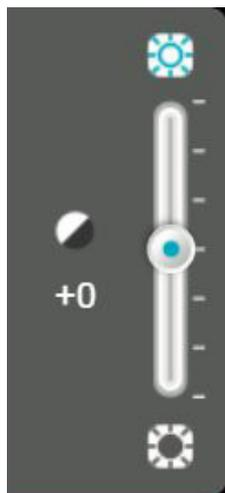
Use the **Exposure** control to adjust the level of exposure. Press the and icons to adjust the level of exposure in increments of 1, between -7 and +7. Exposure can also be adjusted using the slider by left-clicking on and dragging the mouse either up or down.
